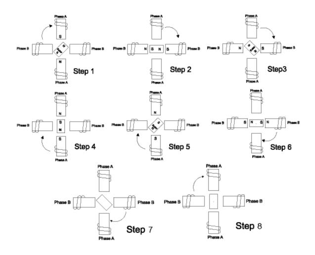
However, half stepping typically results in a 15%-30% loss of torque depending on step rate when compared to the two phase on stepping sequence. Since one of the windings is not energized during each alternating half step there is less electromagnetic force exerted on the rotor resulting in a net loss of torque
